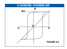
As an example, provided the current transformer under test produces at least 50% of secondary current, a series secondary resistance is varied gradually from 0.1 to 8 ohms and back to 0.1 ohms at a consistent rate. This operation effectively overburdens the current transformer and demagnetizes the core.
