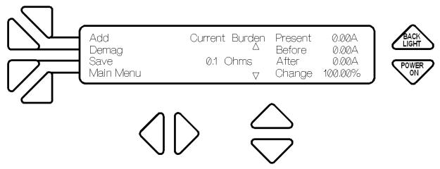
From this screen choose **Demag** by selecting the F2 button and the automatic demagnetization sequence will begin. A sequence of relay clicks about every second for about 7 seconds will be heard during the demag cycle and the following screen will be displayed.
