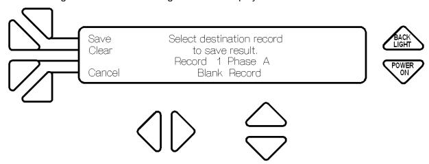
Select the destination record by pushing the ▲ ▼ buttons and push F1 button to *Save* the test results to the record. Press F2 to *Clear* any previous test results in the record. Press F4 to *Cancel* the save and return to the CT Ratio screen.
