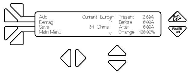
Select the **Burden** value to be added by using the  $\blacktriangle \blacktriangledown$  buttons. To add a burden push F1 to the left of **Add** on the display. The following screen will display.
