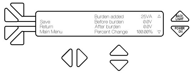
Test data for the various burdens can be viewed by using the  $\blacktriangle \lor$  buttons. To save the data, select the Burden Added value to be saved using the  $\blacktriangle \lor$  buttons and push F2 button to **Save** and the following screen will display. To **Return** to the PT Burden menu without saving the data, push the F3 button. To return to the **Main Menu**, push the F4 button.
