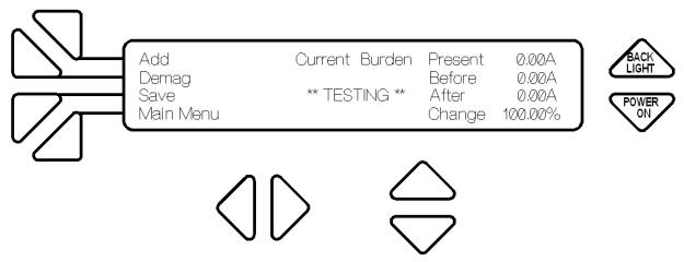
The Before value is the CT secondary loop current just before the burden was applied, the After value is the CT secondary loop current after the burden was applied and the Change is the % of current change between the Before and After CT secondary loop currents. It is left to the user to determine acceptable % of change levels relative to the specific application, selection of CT, and circuit designs of the utility.
