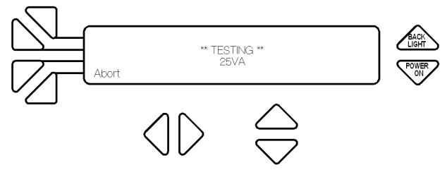
During the test, the screen above will display and a sequence of relays will click every second for about 6 seconds. The value being tested will display on the screen. The burden values are 25, 50, 75, 100, 125, 150 and 175 VA. Push F4 to *Abort* (stop) the test and return to the PT Burden menu screen.
