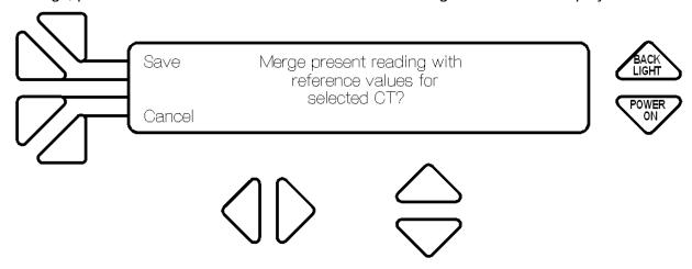
Push F1 button to **Save** the admittance reading or F4 to **Cancel** the save. The 505 will save the last 9999 readings and present the lowest reading for the Minimum, the average of all values for the Average and highest reading for the Maximum. These values are presented for the user to make better decisions about the current admittance reading. When the reading is saved, the display reverts back to the admittance display.
