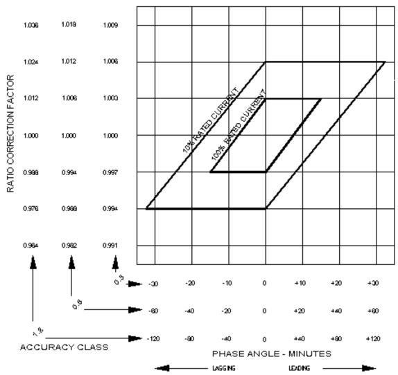
The accuracy requirements for 100% rated current also apply at the continuous-thermal-current rating of the transformer.
