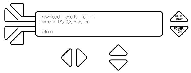
Connect the 9 pin RS-232 cable between the Model 505 panel plug and a selected COM port on the PC loaded with the Results Viewer software. Start the Results Viewer software and select the COM port to which the RS-232 cable is attached. Select the 'Com Settings' tool bar button and choose the COM port from the drop down list.
