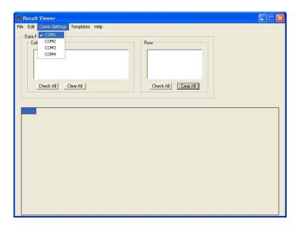
With the RS-232 cable connected and the correct COM port selected, push F1, **Download Results To PC** to begin the download.
