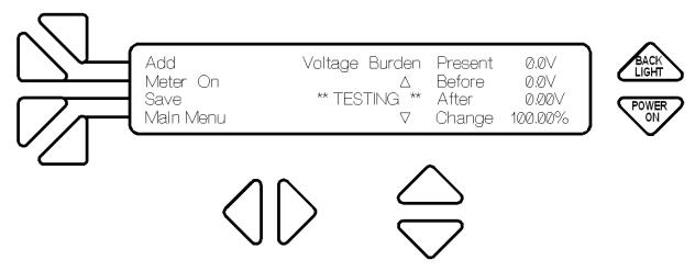
When the test is complete, the Before, After and Change values are displayed. The Before value is the PT secondary voltage just before the burden was applied, the After value is the PT secondary voltage after the burden was applied and the Change is the % of voltage change between the Before and After PT secondary voltages. It is left to the user to determine acceptable % of change levels relative to the specific application, selection of PT, and circuit designs of the utility.
