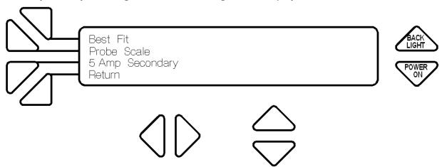
Pushing F1 will select the CT Ratio display to be either **Best Fit** or **Actual**. Selecting F3 will select for the CT Ratio to be calculated using a 5 amp or 1 amp secondary. Selecting F2, **Probe Scale**, will display the following screen.
