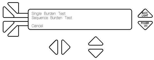
Push the F1 button *Single Burden Test* to add the selected burden. When the F1 button is pushed, the sound of a relay clicking is heard, the following screen is displayed showing that the 505 is \*\*TESTING\*\*.
