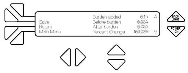
Test data for the various burdens can be viewed by using the  $\blacktriangle \lor$  buttons. To save the data, select the Burden Added value to be saved using the  $\blacktriangle \lor$  buttons and push F2 button to **Save**. and the following screen will display. To **Return** to the CT Burden menu without saving the data, push the F3 button. To return to the **Main Menu**, push the F4 button.
