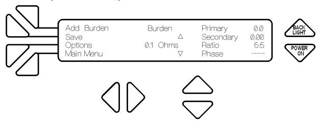
This screen displays that a burden value of 0.1 ohm is selected and will display the Primary, Secondary, Ratio and Phase difference between primary and secondary. Push F1 to *Add Burden* that is selected. The measured values will change displaying the new values with the burden added to the CT secondary loop. To change the burden value, use the ▲ ▼ buttons. The ratio will display calculated as selected in the Options menu – Actual or Best Fit.
