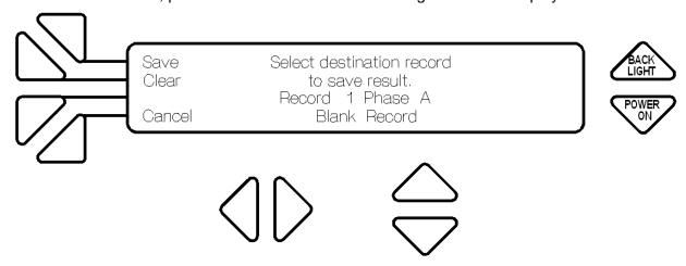
Select the destination record by pushing the ▲ ▼ buttons and push F1 button to **Save** the test results to the record and return to the screen above. Press F2 to **Clear** any previous test results in the record. Press F4 to **Cancel** the save and return to the CT Burden menu screen.
