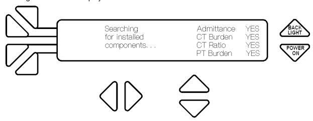
The back light also comes ON during the search. This display indicates that the instrument has the CT/PT Burden Option installed. NO would appear where the YES is now if this option was not installed. This display times out and the following screen is displayed.
