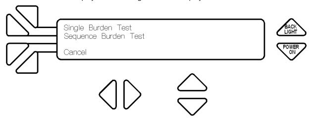
Select **Single Burden Test** by selecting the F1 button, the sound of a relay clicking is heard, the display says \*\*TESTING\*\* and the Before, After and Change values are displayed when the test completes.
