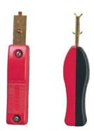
This CT safety test probe is made by Superior and is ½" across. This probe fits most CT test switches but will not fit mini-CT test switches used in sub-station panels.
