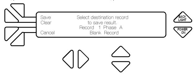
Select the destination record by pushing the ▲ ▼ buttons and push F1 button to *Save* the test results to the record and return to the screen above to select another Burden Value to be saved, etc., until all of the Burden Values are saved. Press F2 to *Clear* any previous test results in the record. Press F4 to *Cancel* the save and return to the CT Burden menu screen.
