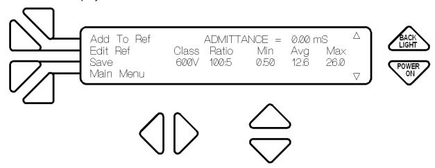
Using the ◀ ▶ and ▲ ▼ buttons, select the Class and Ratio of CT transformer to be tested. The Minimum, Average and Maximum Admittance values for this Class and Ratio of CT will be displayed together with the current Admittance reading. The Minimum, Average and Maximum Admittance values are historical average values based on past measurements for this Class
