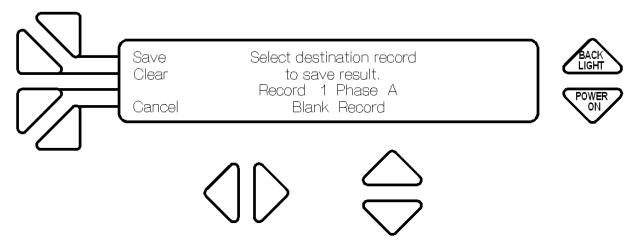
Select the destination record by pushing the ▲ ▼ buttons and push F1 button to *Save* the test results to the record and return to the screen above to select another Burden Value to be saved, etc., until all of the Burden Values are saved. Press F2 to *Clear* any previous test results in the record. Press F4 to *Cancel* the save and return to the PT Burden menu screen.
