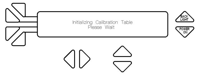
If the *Int Cal Table* button is accidentally pushed, the original factory calibration values that were shipped with the instrument must be re-entered in the *Calibrate* (F3) screen or a new calibration must be made and entered in the *Calibrate* screen. If the original calibration information is unavailable, call Radian Research to request a copy.
