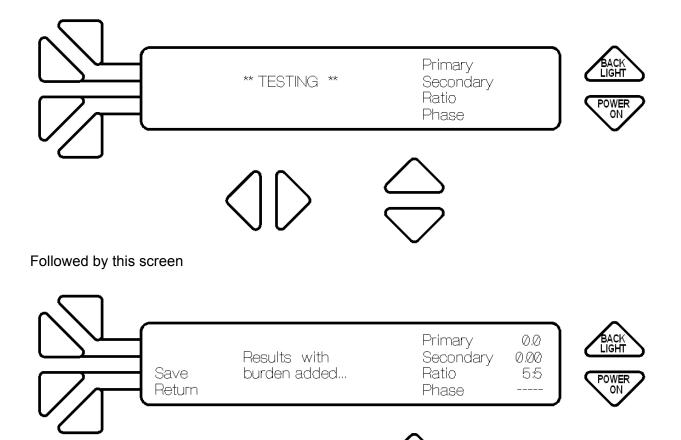
Push F3 to *Save* to display the following screen. Push F4 to *Return* to the CT Ratio screen without saving the data. The following screen will display when the *Save* button is selected.
