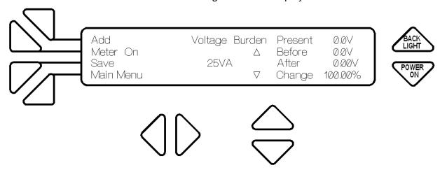
Select the Voltage Burden value to be added by using the  $\blacktriangle \blacktriangledown$  buttons. To add the burden push F1 to the left of *Add* and the following screen will display.
