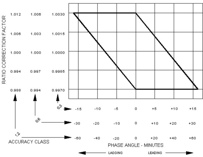
The transformer characteristics shall lie within the limits of the parallelogram for all voltages between 90% and 110% of rated voltage.
