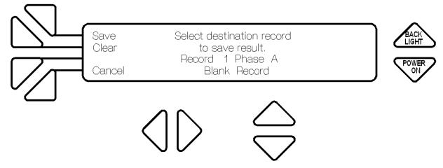
Select the destination record by pushing the ▲ ▼ buttons and push F1 button to **Save** the test results to the record. Press F2 to **Clear** any previous test results in the record. Press F4 to **Cancel** the save and return to the PT Burden menu screen.
