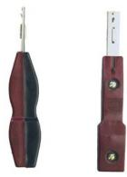
This CT safety test probe is made by Westinghouse and is about 3/8" across. This probe fits most CT test switches and mini-CT test switches. It is not as rugged as the Superior and is easily damaged.
