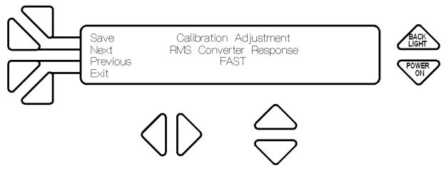
The RMS Converter Response can be set from SLOW, MED and FAST. SLOW is the longest sample time and produces the most accurate readings. The settling time can be shortened at the expense of accuracy in the measurements. The factory default setting for the RMS Converter Response is FAST. Press F1, *Save* after making any changes in the Calibrate screen.
