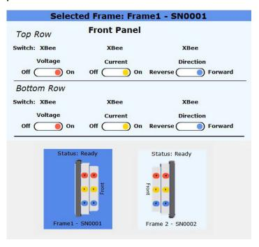
Further flexibility is achieved by enabling local override to the XBee controls. Each WECO SMART AMI Meter Farm row of meters can be set to disable the remote XBee control mechanism preventing any non-local changes.
