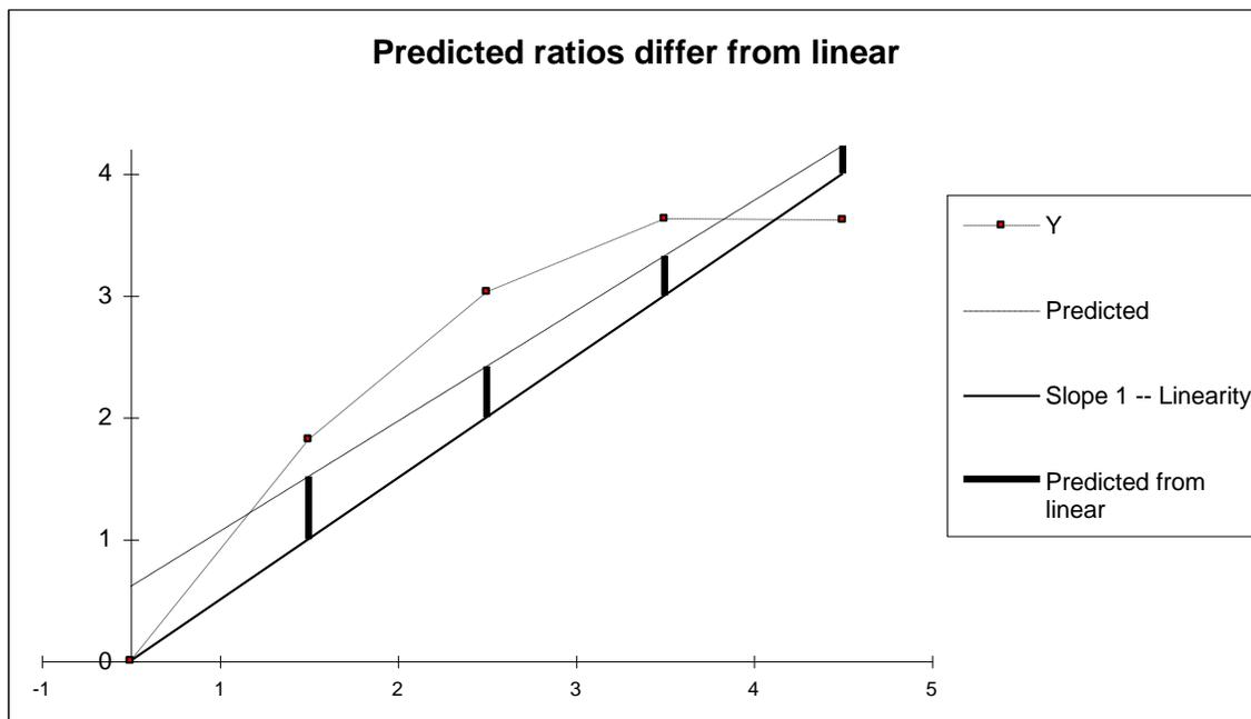
Figure 5 -- Plot of least-squares fit showing the errors between the Predicted Ratios and the Nominal Ratios (slope=1)
