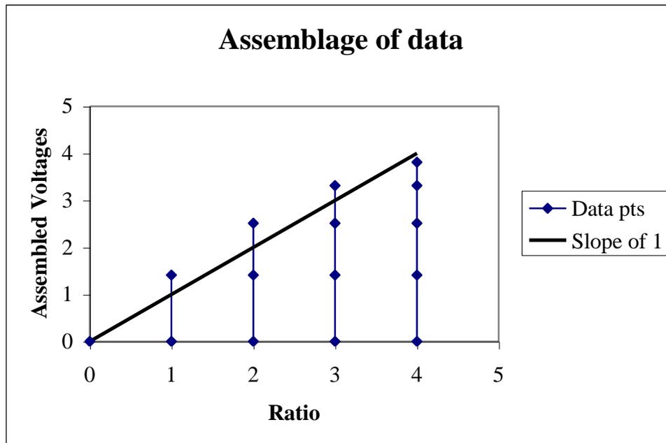
Figure 1 -- Assembled calibration data formed by combining the incremental measurements.
