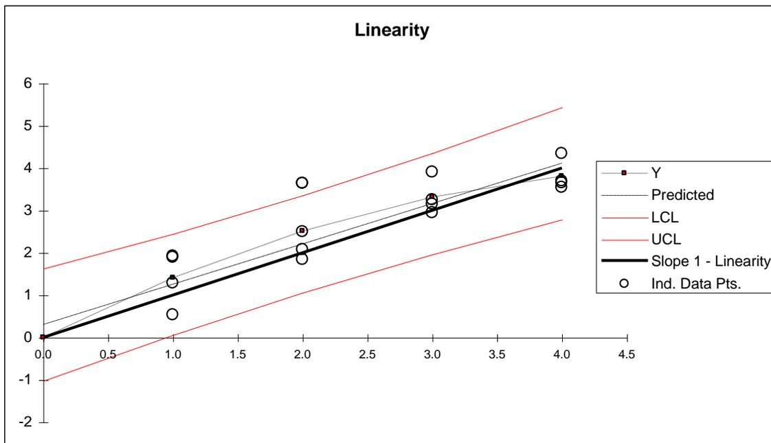
Figure 2 -- Least-squares curve fit demonstrating non-linearity and repeatability in the measuring system showing the Upper and Lower Control Limits (LCL and UCL) set at 95% confidence.
