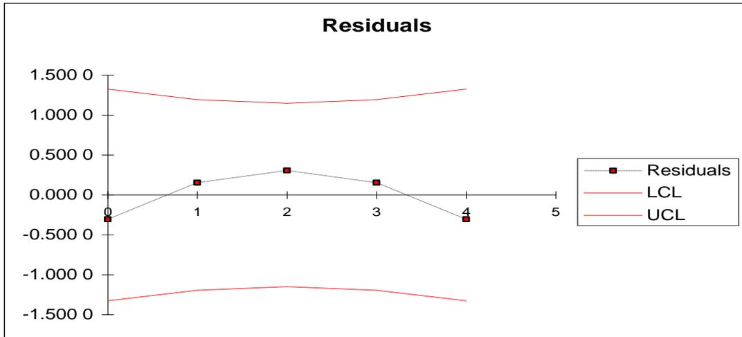
Figure 3 -- The residuals from the curve fit showing significant non-linearity
