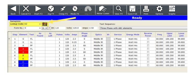
Now we can look at another feature which is barcoding. Barcodes have been used for many years by the utility industry to help define and track equipment. Barcoding made its way into meter testing to speed up testing and help prevent data entry mistakes caused by manually typing in data.
