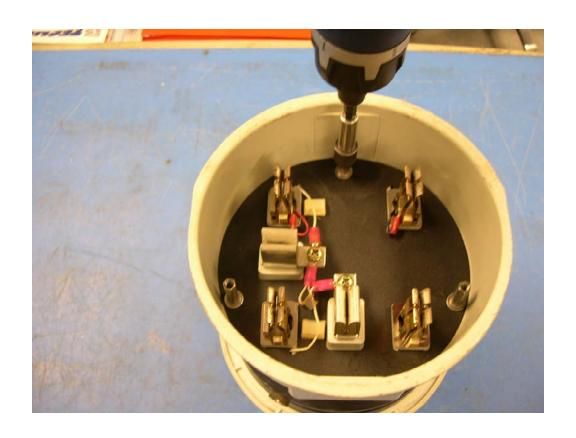
4. Carefully remove the chassis from the socket base.
