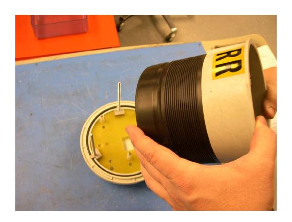
5. Replace the internal fuses as necessary.
